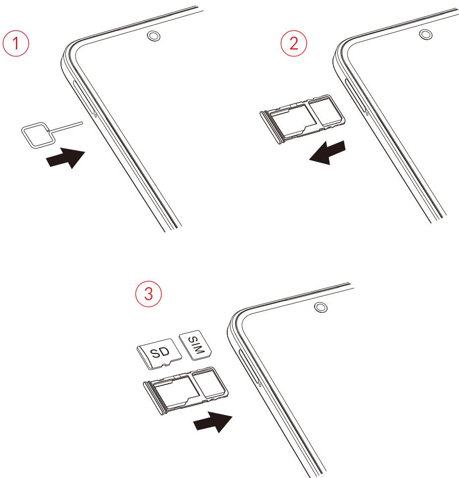
You must insert your SIM card to make phone calls. You do not need to power off your phone before inserting or removing the SIM card as this phone supports hot swap.
